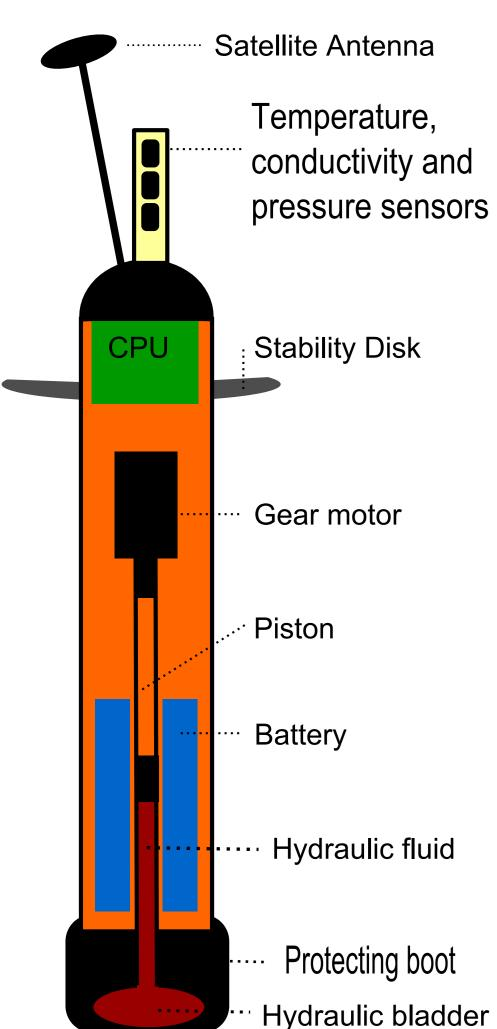
Argo floats are robotic devices that are deployed from ships or planes and that freely drift in the ocean over a typical period of 5 years. These floats pump fluid from an external bladder towards the interior of the float. This pumping action reduces the volume of water displaced by the float and, through Archimedes' principle, this makes the float denser allowing it to sink to a predetermined depth such as 1000 m or 2000 m.
