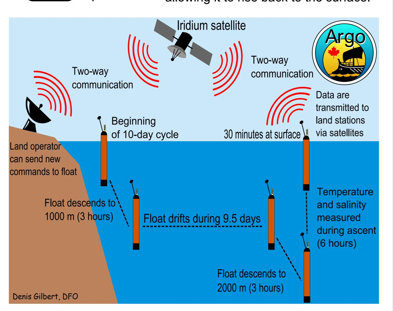
Early models of Argo floats used one-way communication, meaning that while we could receive data from the floats, we could not send confirmation to the float that we had received its data and we could not change the float's mission parameters once it was deployed. Newer models now take advantage of two-way communication capability and a much faster data flow, which allows us to reduce time spent by the float on the surface to merely 30 minutes compared to 6 hours in earlier models.
